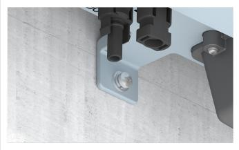
5. Rehang the inverter and fasten the screws on the underside.
