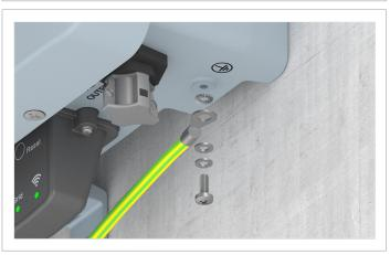
6. Bolt the grounding cable onto the inverter. Nut, spring washer, washer, and toothed lock washer are already mounted on the inverter.
