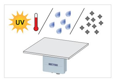
▶ The inverter has a protection degree of IP65 and can be installed indoors and outdoors. Despite this, the inverter should be protected by a roof against direct solar irradiation, rain and snow. For example, the power of the inverter will be reduced if it is too heavily heated by solar radiation. This is normal operating behavior for the inverter and is necessary to protect the internal electronics.
