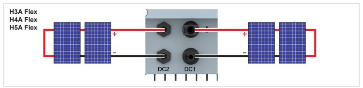
Connect the negative pole of the solar module string to DC–, connect the positive pole to DC+.
