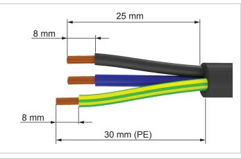
1. Remove the insulation from the cable and wires. Do not twist the wire ends because this reduces the contact surface area with the wire end sleeves.
