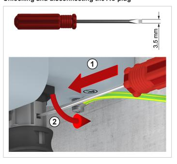
➤ To disconnect the AC plug from the inverter, use a screwdriver to push down the locking mechanism on the AC socket.
