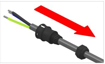
5. Unscrew the nut and housing over the cable.
