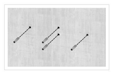
1. Attach the mounting plate to the wall/the mounting system using 4 M6 screws and washers.
